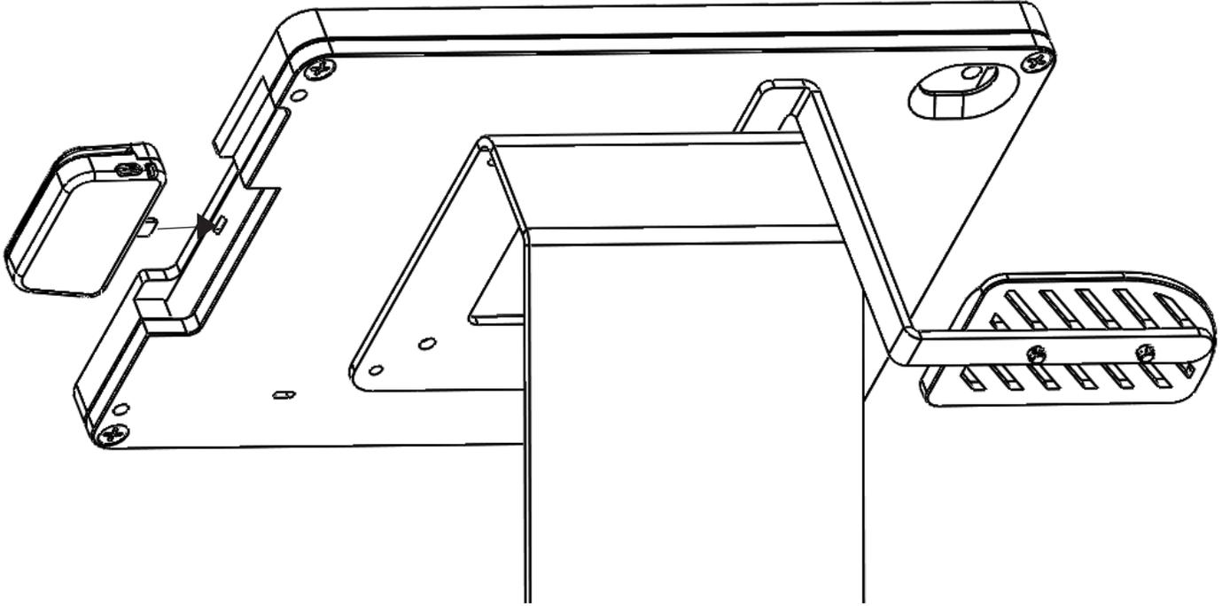
④ Install the ID TECH iMaG Pro II bracket over top of the card reader
