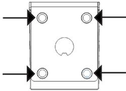
For a non-permanent mounting solution, use the (4) included black rubber hemispheres. Peel off the film and apply each hemisphere to the perimeter of the base as shown above
